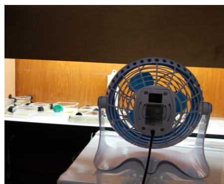
Figure 6 Example of simple "incubator" with ventilation to cultivate microalgae In this example, the fluorescent lights are at the top of the cultures, protecting eyes from bright exposure with a front cover. To reduce temperature, their high heat-producer reactants may be installed far away and/or a ventilator installed to the side of the cultures. A white color bottom may be used to reflect light. Light intensity. Light intensity is measured in µmol photon/m 2 /s. A recommended starting value of light intensity to cultivate microalgae may be ~50-100 µmol photon/m 2 /s.
