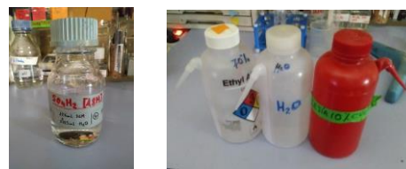
Figure 9 Example of a highly toxic chemical and easy dispensable liquids. A crystal bottle to hold 20-fold diluted corrosive sulfuric acid SO 4 H 2 and 500 mL flasks for 70 % ethanol (to disinfect hands), distilled water, and 10 % bleach (to disinfect surfaces).
